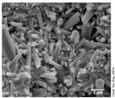
Figure 3. Surface microstructure of bioactive  $Si_3N_4$ .
