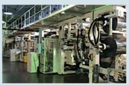
EMC plans to fabricate the panels on its high-speed, roll-to-roll manufacturing lines.
