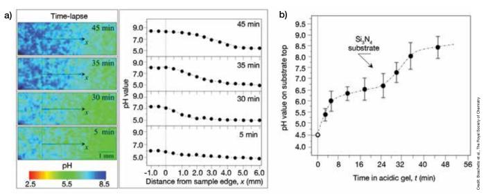
Figure 2. a) Evolution of pH near a silicon nitride surface when placed in an acidic gel; b) average surface pH over time for same experiment. Republished with permission from The Royal Society of Chemistry, from Boschetto et al.<sup>5</sup>; permission conveyed through Copyright Clearance Center, Inc.
