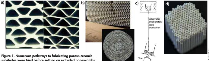
substrates were tried before settling on extruded honeycombs. (a) Alternate layers of flat and crimped paper infused with glass-
