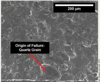
Figure 1. The fractographic technique is used to observe failure points, as shown in this SEM-micrograph of a large quartz grain at tensile surface.
