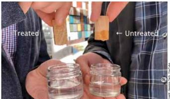
By treating wood using atomic layer deposition, Georgia Tech researchers found they could manage moisture content, mold growth, and thermal conductivity.
