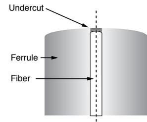
Figure 3. Fiber Undercut | Drawing ZA-1269
