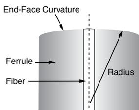
Figure 1. Radius of Curvature
