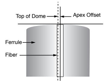
Figure 2. Apex Offset | Drawing ZA-1269
