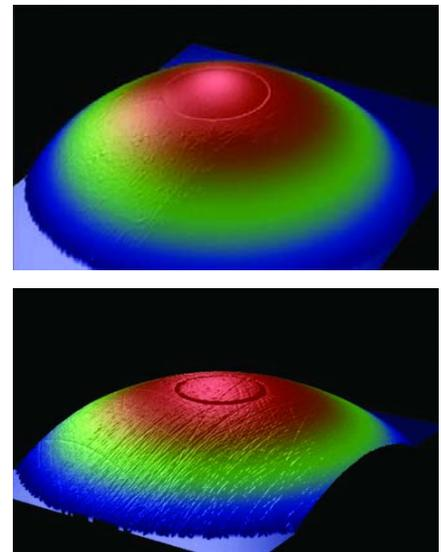
Figure 4. In the top image (a three-dimensional image of a UniCam Connector ferrule), fiber undercut has been precisely maintained to create a nearly smooth end-face. The factory-controlled polish leaves the surface nearly perfect. In the bottom image, this anaerobic connector ferrule end-face shows visible fiber protrusion and the hand polish has resulted in scratches over the entirety of the end-face.
