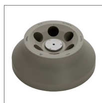
6 x 50 mL fixed angle rotor (Cat. No. 480136)
